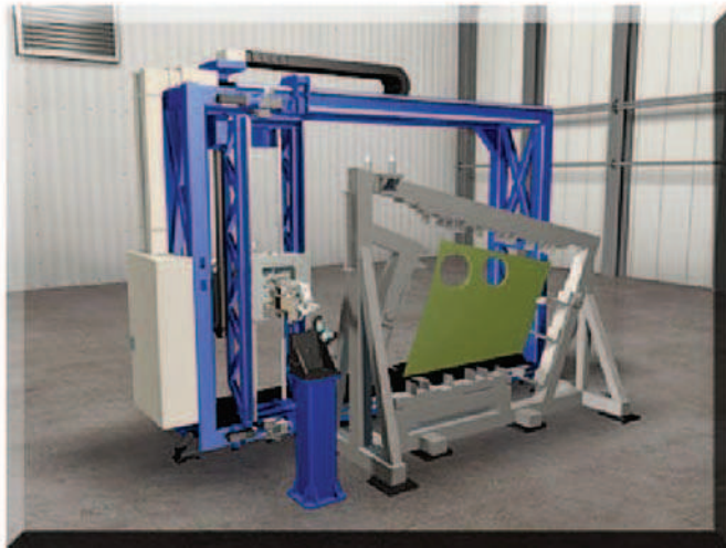
Fig. 11.17. Outer Wing NCDJ Drilling System 10
