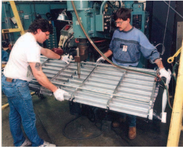
Fig. 9.28. Spot Welding TMC Hat Stiffeners Source: The Boeing Company
