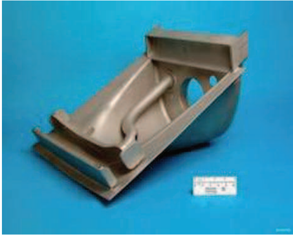
Fig. 4.25. Titanium Investment Casting Source: The Boeing Company
