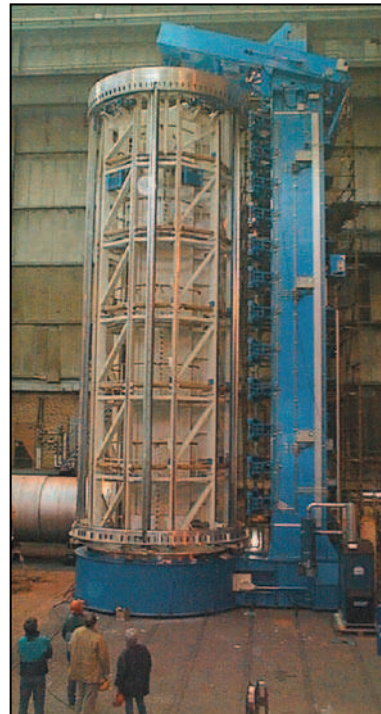
Fig. 2.46. Friction Stir Welding Applications for Delta Source: ESAB Welding Equipment AB and The Boeing Company
