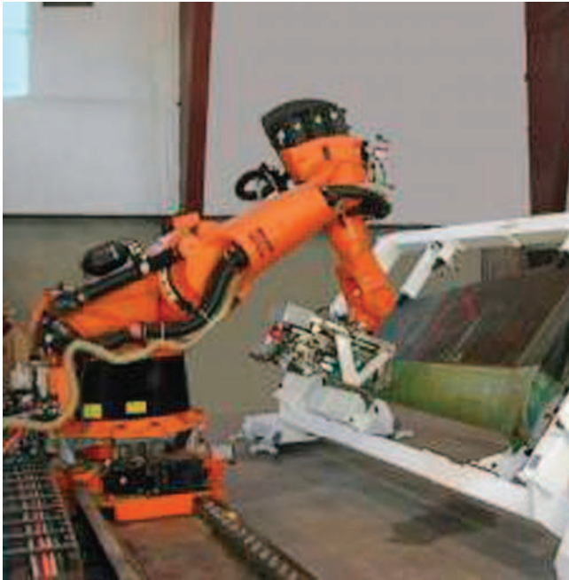
Fig. 11.15. Robotic Drilling of Control Surface Source: The Boeing Company
