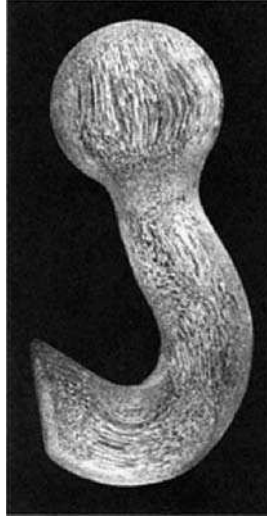
Fig. 5.10. Etched 4140 Forging Showing Grain Flow 7
