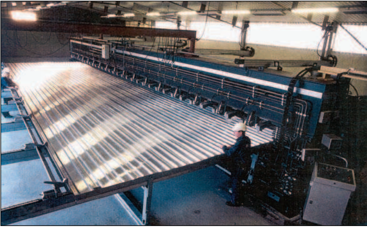
Fig. 2.47. Large Friction Stir Welder Being Used in Marine Industry Source: ESAB Welding Equipment AB
