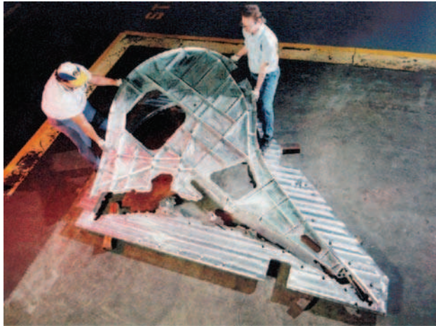
Fig. 2.33. High Speed Machined Unitized Bulkheads Source: The Boeing Company
