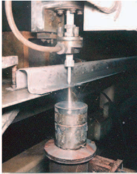
Fig. 9.25. Abrasive Waterjet Cutting of TMC Source: The Boeing Company
