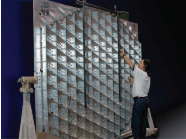
Fig. 2.31. High Speed Machined Thin Wall Space Structure Source: AUT Inc.
