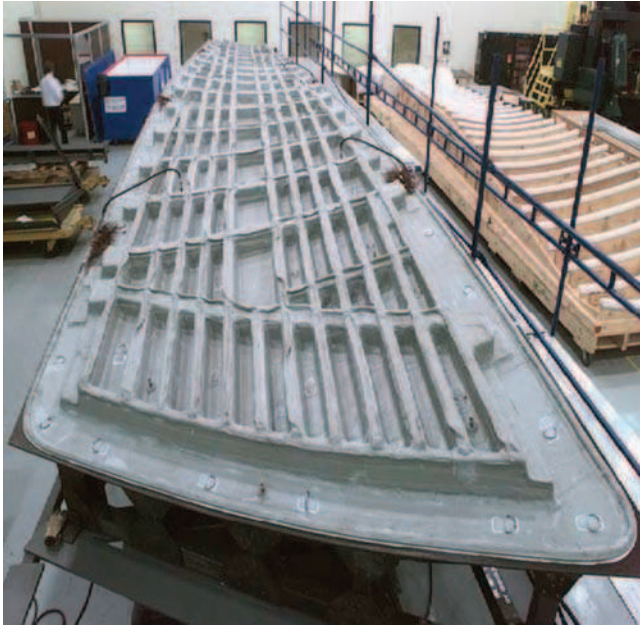
Fig. 7.28. Large Reusable Silicone Rubber Vacuum Bag Source: The Boeing Company
