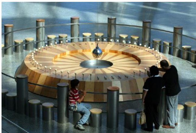
Figure 4.1.3: As Earth turns, the plane of oscillation of the Foucault pendulum shifts gradually so that over the course of 12 hours, all the targets in the circle at the edge of the wooden platform are knocked over in sequence.
