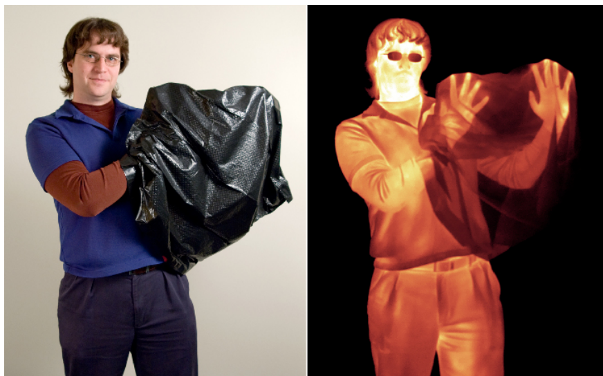
Figure 6.3.2: Infrared Eyes. Infrared waves can penetrate places in the universe from which light is blocked, as shown in this infrared image where the plastic bag blocks visible light but not infrared.
