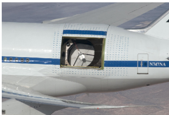
Figure 6.5.1 Stratospheric Observatory for Infrared Astronomy (SOFIA). SOFIA allows observations to be made above most of Earth's atmospheric water vapor.
