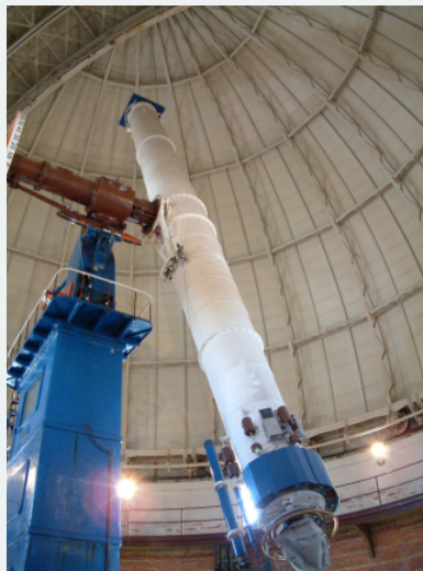
Figure 6.2.5 World’s Largest Refractor. The Yerkes 40-inch (1-meter) telescope.
