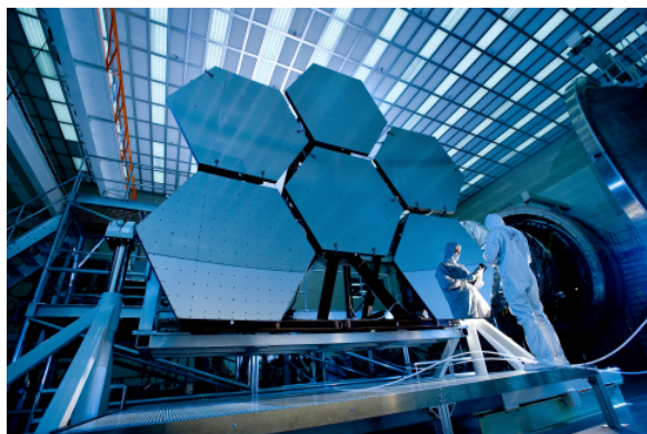
Figure 6.6.1 James Webb Space Telescope (JWST). This image shows some of the mirrors of the JWST as they underwent cryogenic testing. The mirrors were exposed to extreme temperatures in order to gather accurate measurements on changes in their shape as they heated and cooled. (credit: NASA/MSFC/David Higginbotham/Emmett Given)
