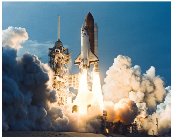
Figure 3.2.2 Demonstrating Newton's Third Law. The U.S. Space Shuttle (here launching Discovery), powered by three fuel engines burning liquid oxygen and liquid hydrogen, with two solid fuel boosters, demonstrates Newton's third law. (credit: modification of work by NASA)
