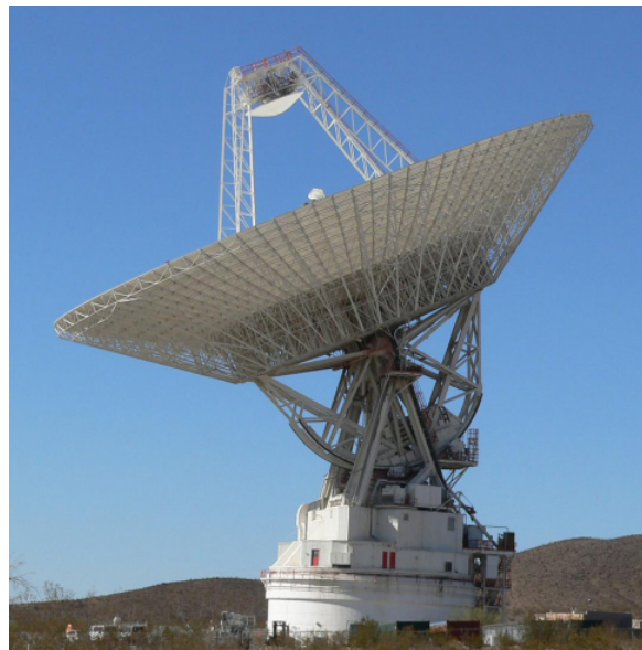
Figure 19.1.2 Radar Telescope. This dish-shaped antenna, part of the NASA Deep Space Network in California’s Mojave Desert, is 70 meters wide. Nicknamed the “Mars antenna,” this radar telescope can send and receive radar waves, and thus measure the distances to planets, satellites, and asteroids.
