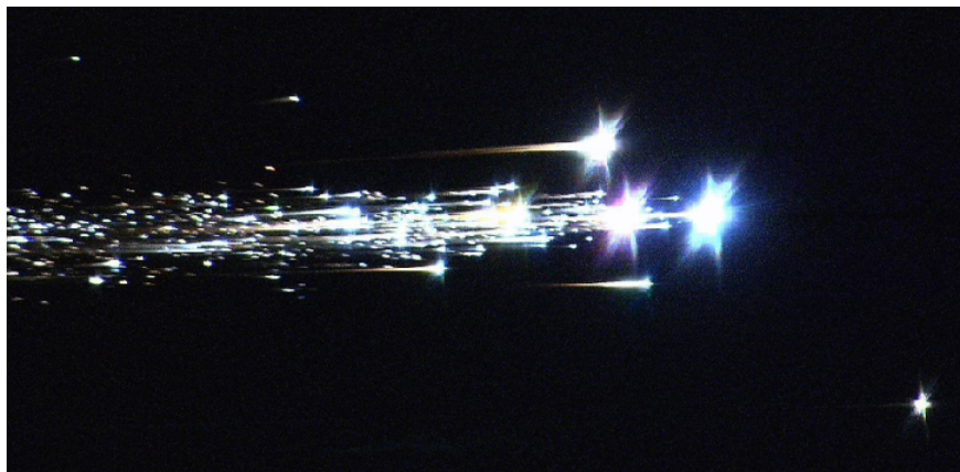
Figure 13.1.9 Hayabusa Return. This dramatic image shows the Hayabusa probe breaking up upon reentry. The return capsule, which separated from the main spacecraft and parachuted to the surface, glows at the bottom right.
