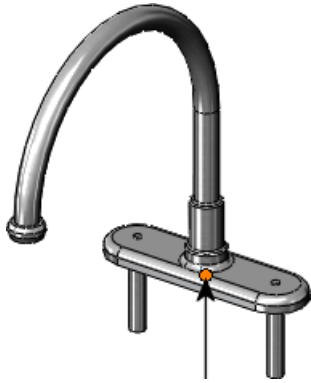
Faucet component with origin (assembly origin and component origin)
